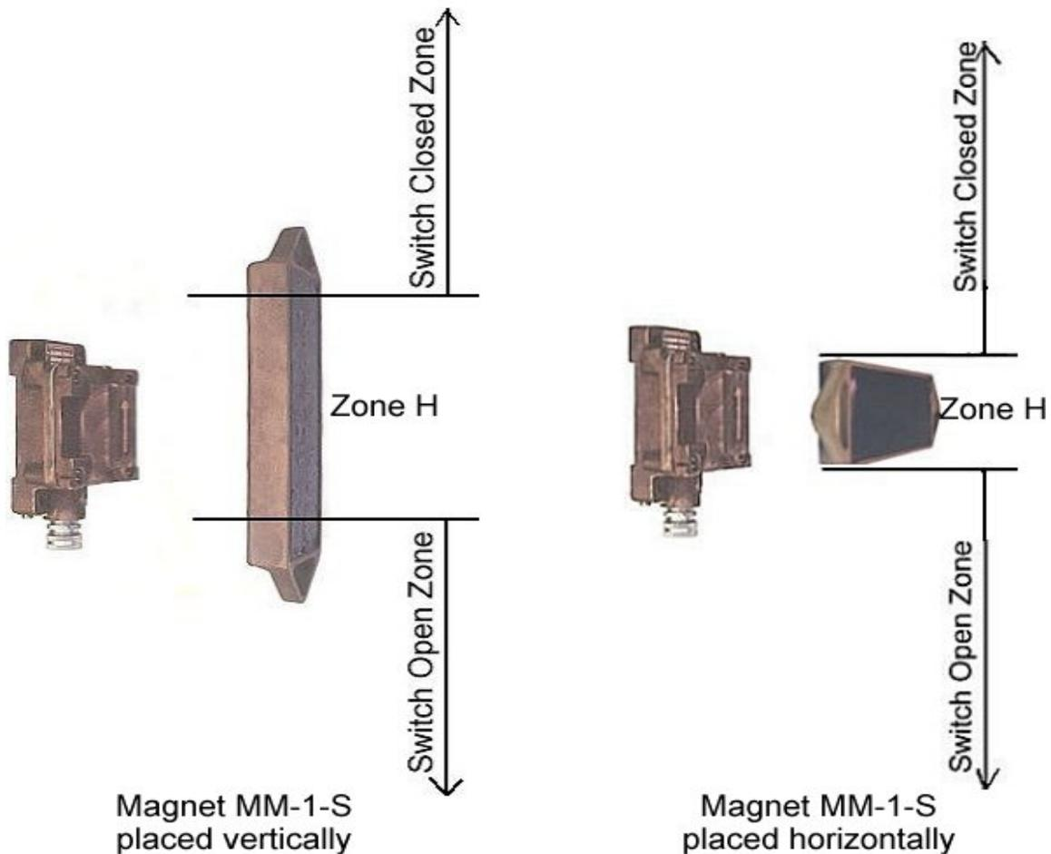
In Zone H, the switch status could be closed or open, depending on the direction of movement. If the magnet is moving down the switch is closed in Zone H and opens when the magnet reaches "Switch Open Zone". If the magnet is moving up, the switch is open in Zone H and closes when the magnet reaches "Switch Closed Zone". Note, that the "undefined" Zone H is wider if the magnet is oriented vertically. So if a narrow Zone H is required, the magnet should be mounted in a horizontal position.
